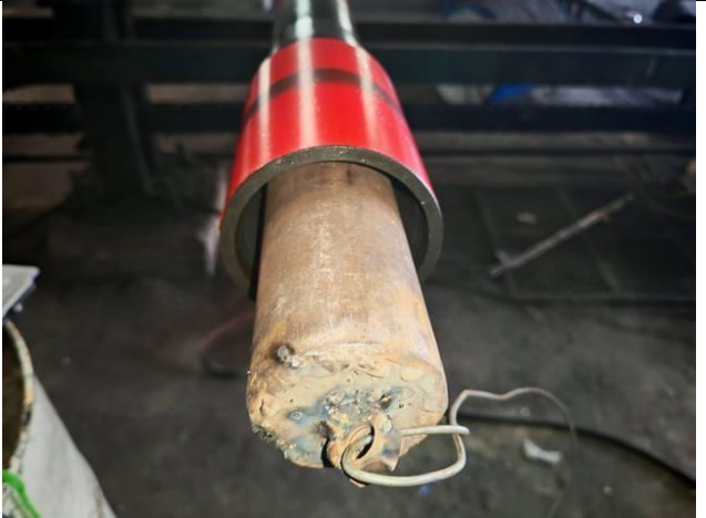
drift test inspection
