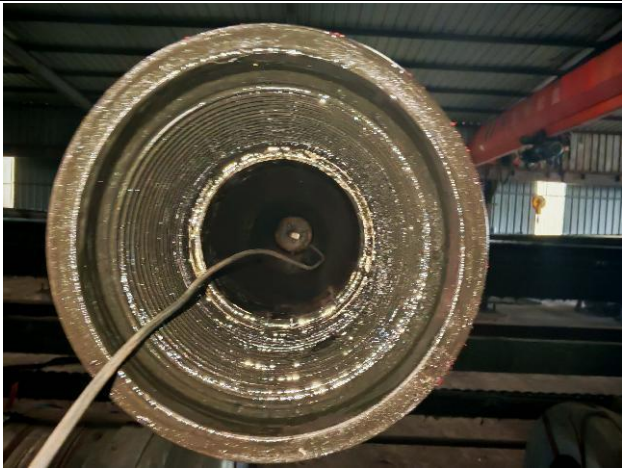
drift test inspection
