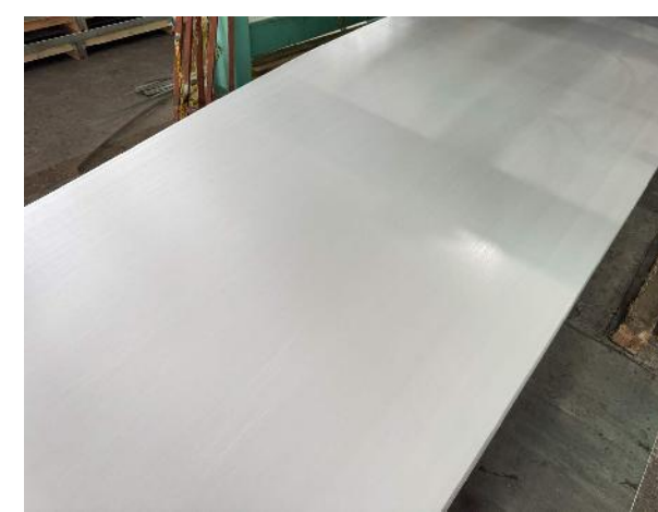
Visual inspection(Plate 1500*3mm*10000mm)
