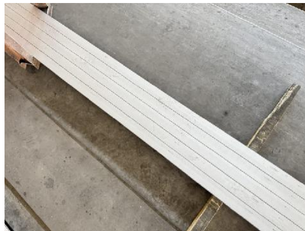
Visual inspection(Flat steel 50*5mm*6000mm)
