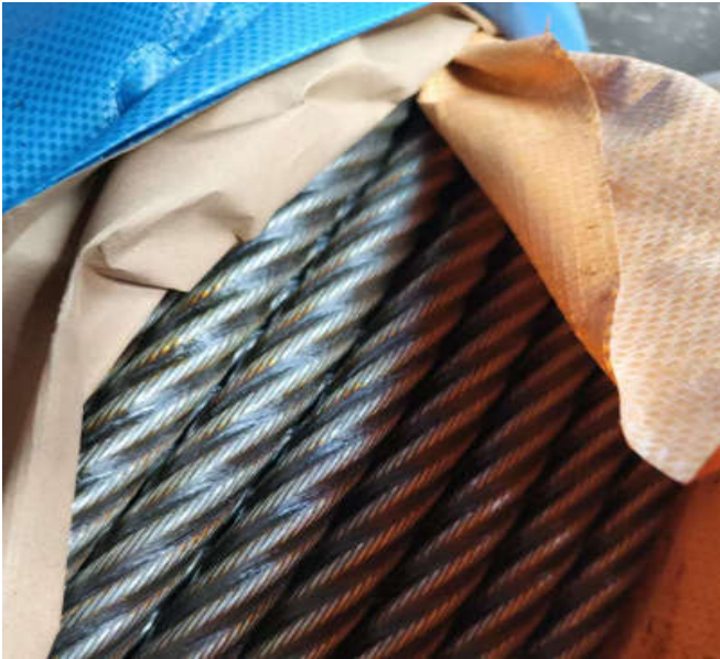
Lay direction of strand and surface lubrication inspection the result complied with order requirement
