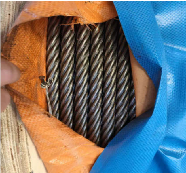
Lay direction of strand and surface lubrication inspection the result complied with order requirement
