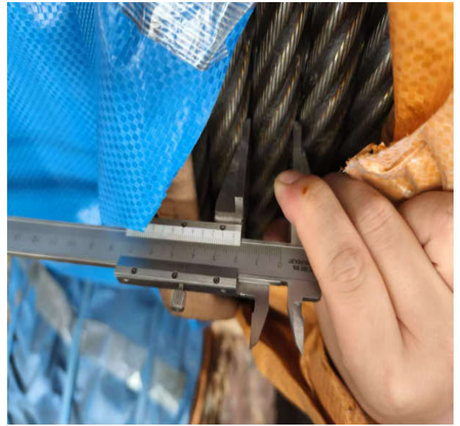
Steel wire rope diameter inspection. the result complied with standard ASTM A1023-09 table 6
