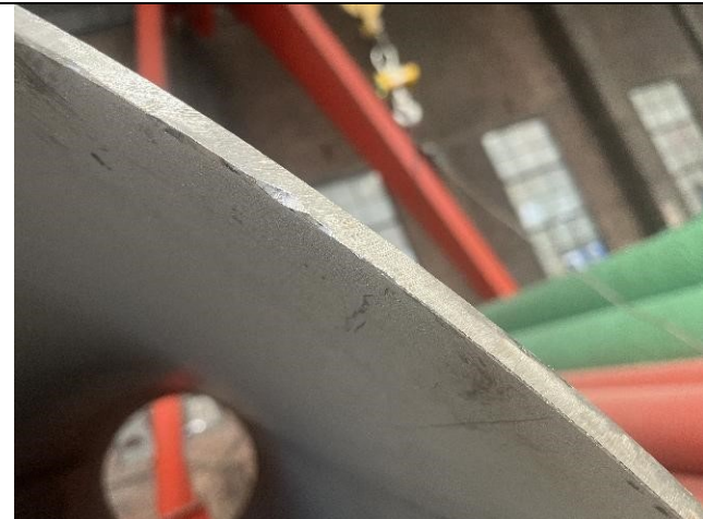
KNOCKED DAMAGE WAS FOUND
