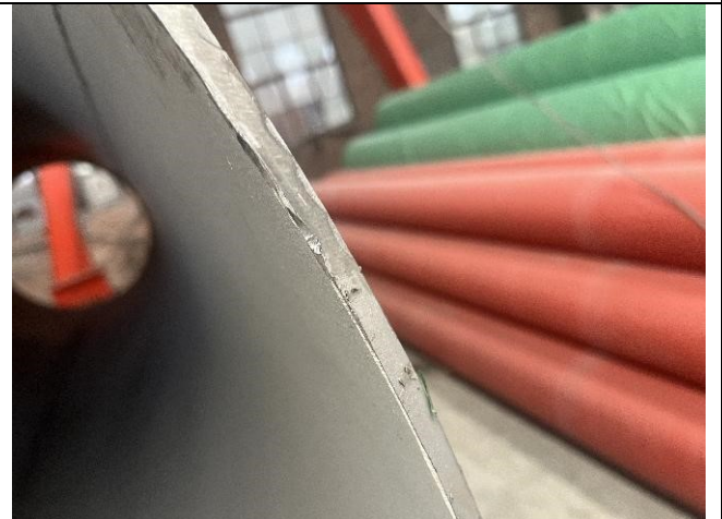
KNOCKED DAMAGE WAS FOUND
