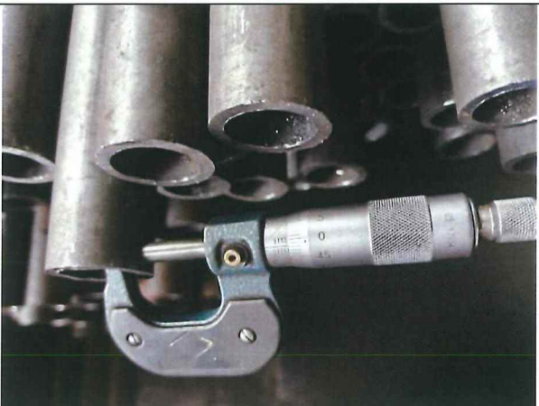
Wall thickness check
