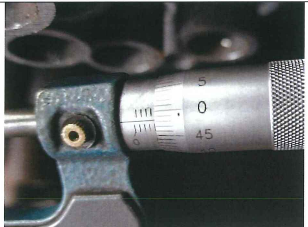
Wall thickness check
